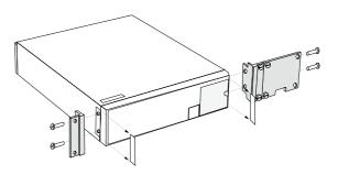
• Fasten the 6688 or 6689 in the rack via screws in the four rack mounting holes
